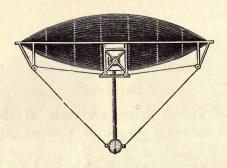
enables their position to be adjusted by means of a hand wheel. A rod which is fulcrumed below the balloon carries a hollow ball at its lower end containing sand, and by adjusting this rod forward or backward the angle of the balloon may be adjusted. By opening a valve at the lower part of the ball, sand may be discharged from same and thus serve the purpose of ballast.
